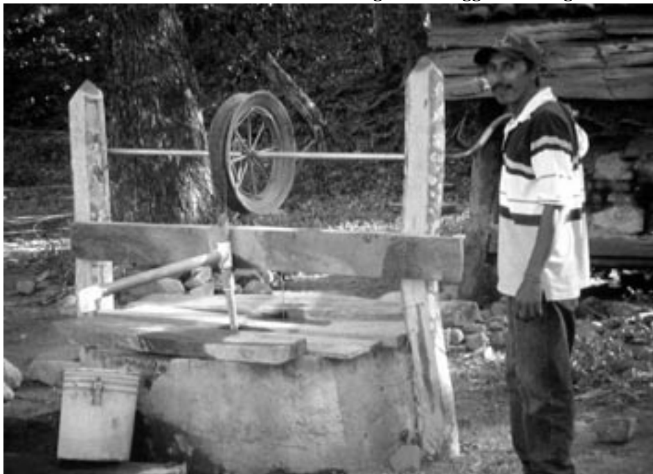
Well with rope pump constructed by the Richland Center-Santa Teresa Sister City Project near La Poma.
